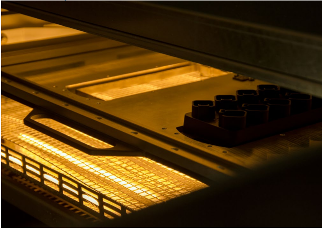
The SMARTFLOW pre-heater with infrared lamp segments.
